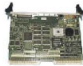
Figure 1: VSH750 750/G4 AltiVec "Hot Swap" Master Controller Single-Board Computer for 6U VME
